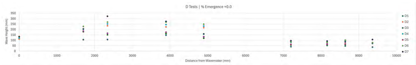
Figure 53. Measured wave height variation along the flume for D tests of the Defender™ model.
